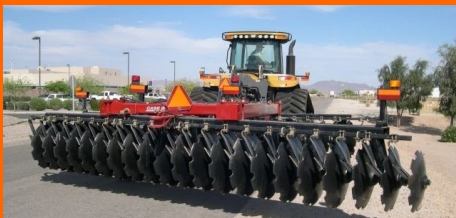
Make sure your equipment has SMV signs and they are visible from behind.
